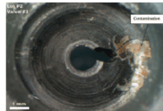
Fig 1.4 — Valve observed during microscopy at 10x magnification. Note the presence of pinkish droplets on the edge of the valve opening, representing gross contamination.
